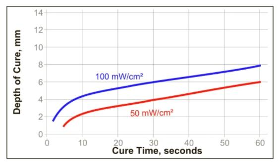
Curing System: Electrodeless, H bulb
