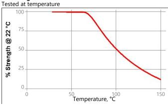
Cured for 5 days @ 22 °C Lap Shear Strength, ISO 4587: Steel
